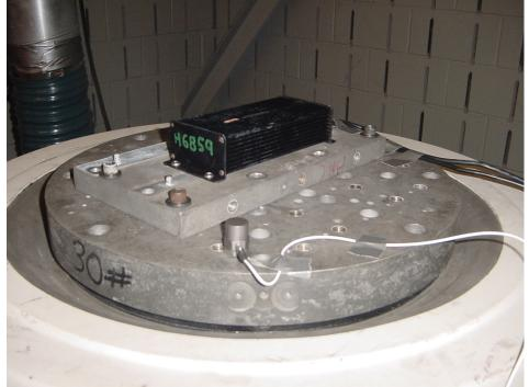
Figure 5: Vertical Functional Shock and Vibration Test Setup
