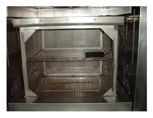
Figure 2: Thermal Shock Test Setup
