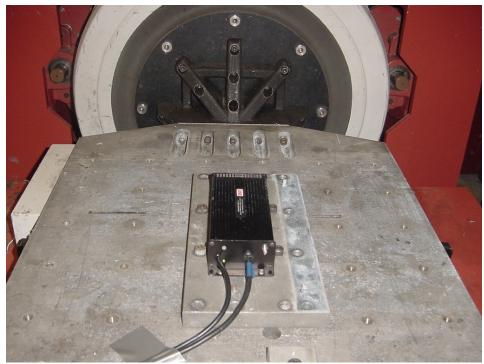
Figure 3: Longitudinal Functional Shock and Vibration Test Setup
